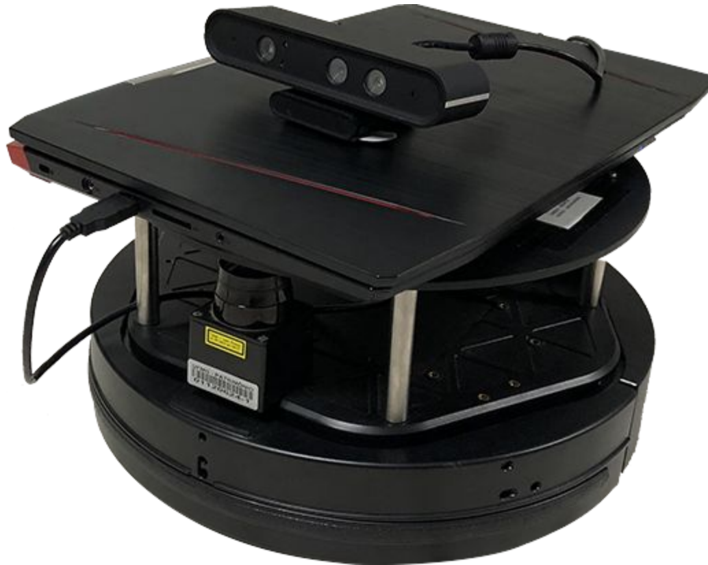
Kobuki Base, RGBD camera, 2D Lidar.
